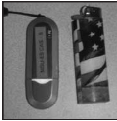
A USB jump drive (sometimes called a pen drive) is about the size of a lighter.
