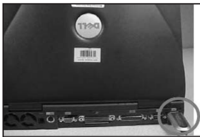
USB pen drive inserted into the USB port on the back of a laptop.
