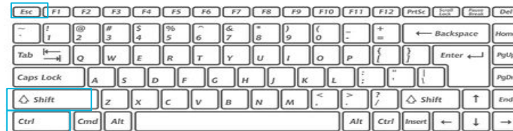
Image of how to access the task manager on a Windows keyboard
